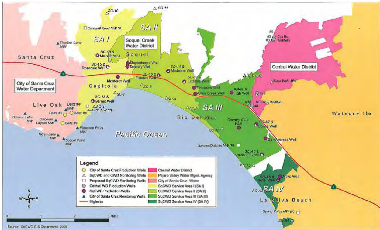
Figure 6-2. Public Water System Production and Monitoring Wells
